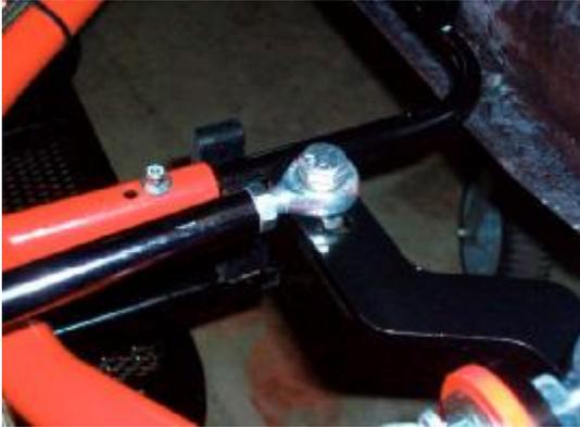
front-end geometry and the rate of speed, the inside tire radius compared to the outside tire. This is based on the theory that the LF tire is traveling on a tighter radius than the RF tire. The 2010 EXCENTRIK has multiple adjustments and from the factory will be in the center positions. With testing, we found that these settings will be the best suited for most track condition; however, these may vary due to track surfaces and conditions.
